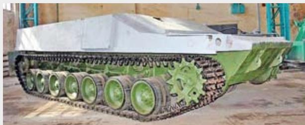
Kharkiv Armor Repair Plant has developed and built a new armored fighting platform that shares power plant and related servicing systems as well as transmission, chassis and electric equipment with the T-80 main battle tank and Oplot tank, Ukraine
