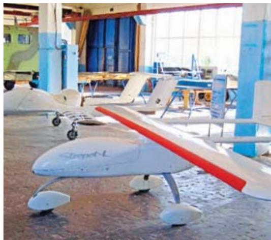
The tactical UAS 'STREPET-L' has a maximum take-off mass of 80 kg, including a 20kg payload. Effective range is put at 80 km and practical ceiling at 4,000m. Fuel endurance is enough for up to four hours in the air at a cruising speed of 130 kph.
