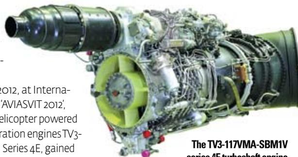
The TV3-117VMA-SBM1V series 4E turboshaft engine for Mi-8 helicopter
