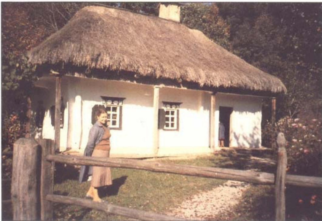
Adobe houses with thatched roofs were once common in the Ukrainian countryside. Photograph by N. Kononenko
